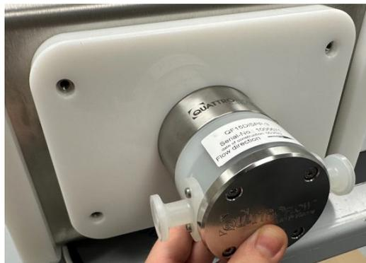
Step 4. Once all four screws are removed, pull the pump head to dismount it from the mounting posts.
