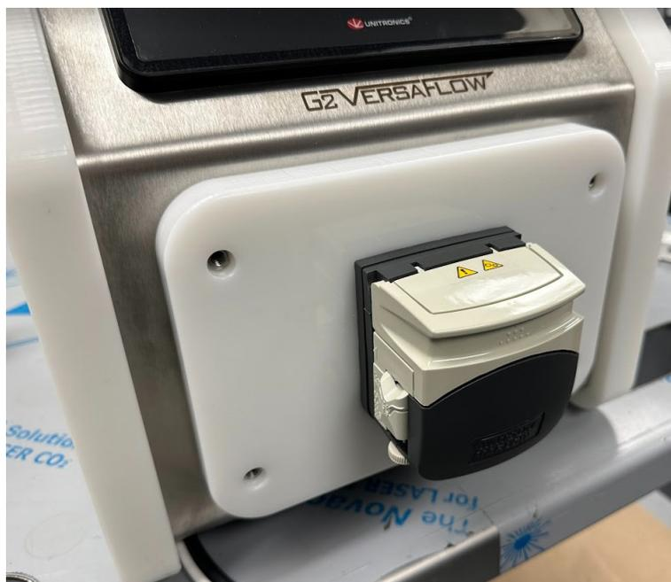
Step 8. Replace the thumbscrews onto the mounting posts to secure the pump head to the OnePump VersaFlow console. Alternate diagonally which screws are fastened. Once all the screws are replaced, check each screw for tightness one more time.
