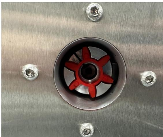
Step 6. Rotate the shaft coupling so that it aligns with the gap in the spider bushing. When assembling a Quattroflow pump head onto the motor, do so without the single-use pump head installed. You may use the center screw on the front of the swash plate to align the pump coupling by hand.
